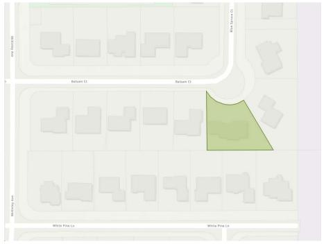
The existing home is located 31'9" from the rear (south) property line at the closest point as measured from the southeast wall of the residence to the property line. The proposed addition is located on the southwest corner of the home. An outline of the proposed setback can be seen below.
