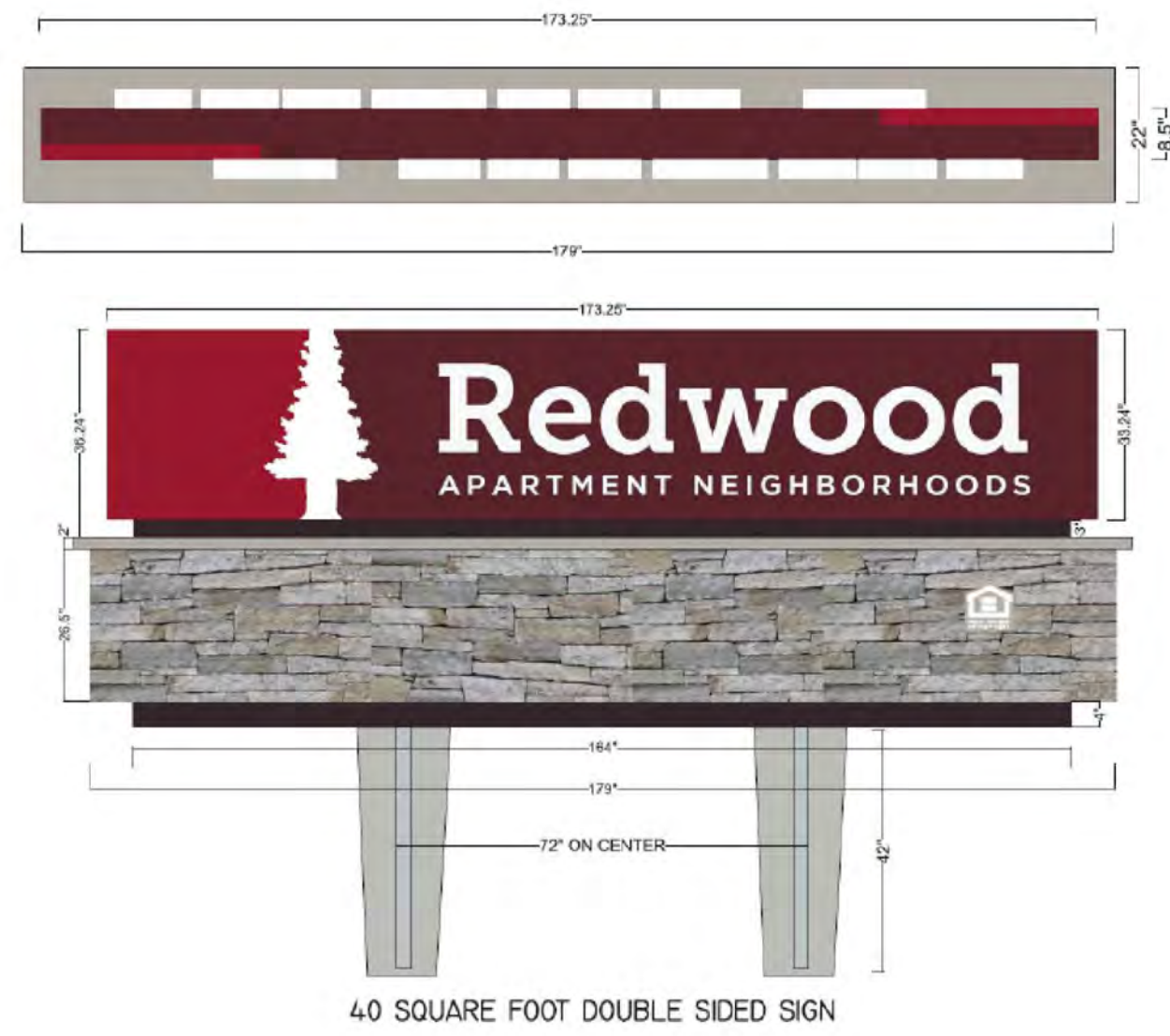
NOTES 1. SIGN SHALL BE DOUBLE SIDED, INTERNALLY ILLUMINATED AND LOCATED PERPENDICULAR TO THE RIGHT OF WAY. MAIN ENTRY SIGN NOT TO SCALE
